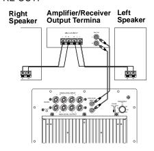
Note: We recommend you connect the subwoofer to an amplifier or receiver that has at least two sets of line out jacks. Connecting the subwoofer to an amplifier or receiver with only one set of line out jacks might result in no sound from the satellite speakers. If your amplifier has only one set of line out jacks, follow the instructions under "Connecting to Speaker Terminals" instead.
